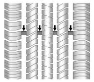
One way to tell when it is time for new tires is to check the treadwear indicators, which appear when the tires have only 1.6 mm (1/16 in) or less of tread remaining. See *Tire Inspection on page 10-51* and *Tire Rotation on page 10-51* for additional information.
